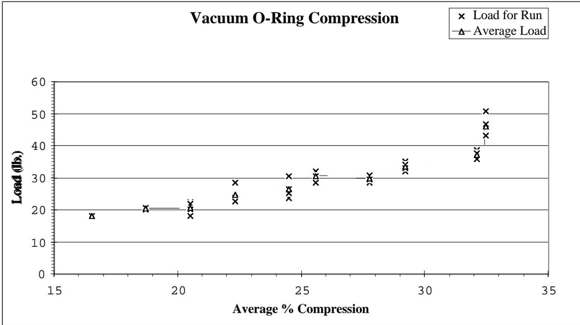
Figure 9. Graph of data from the compression experiment.
