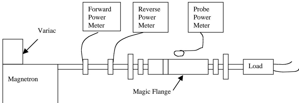
Figure 5. RF Testing Apparatus (layout)
