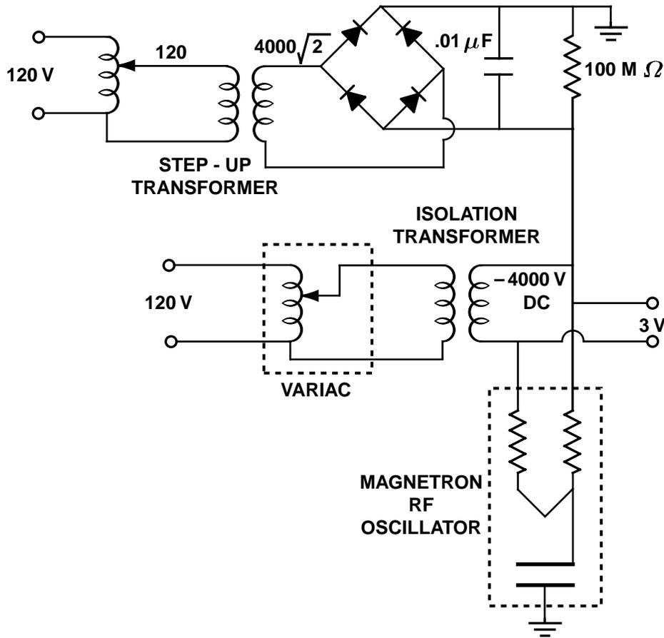
Figure 4. Schematic of the Magnetron Apparatus (circuit).
