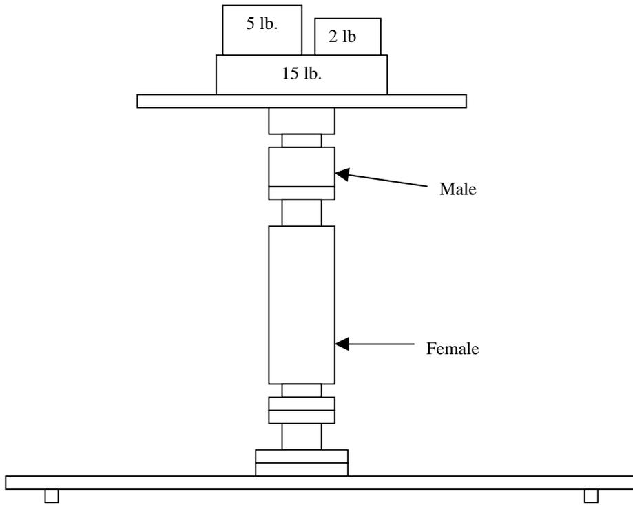
Figure 8. Assembly Force Test
