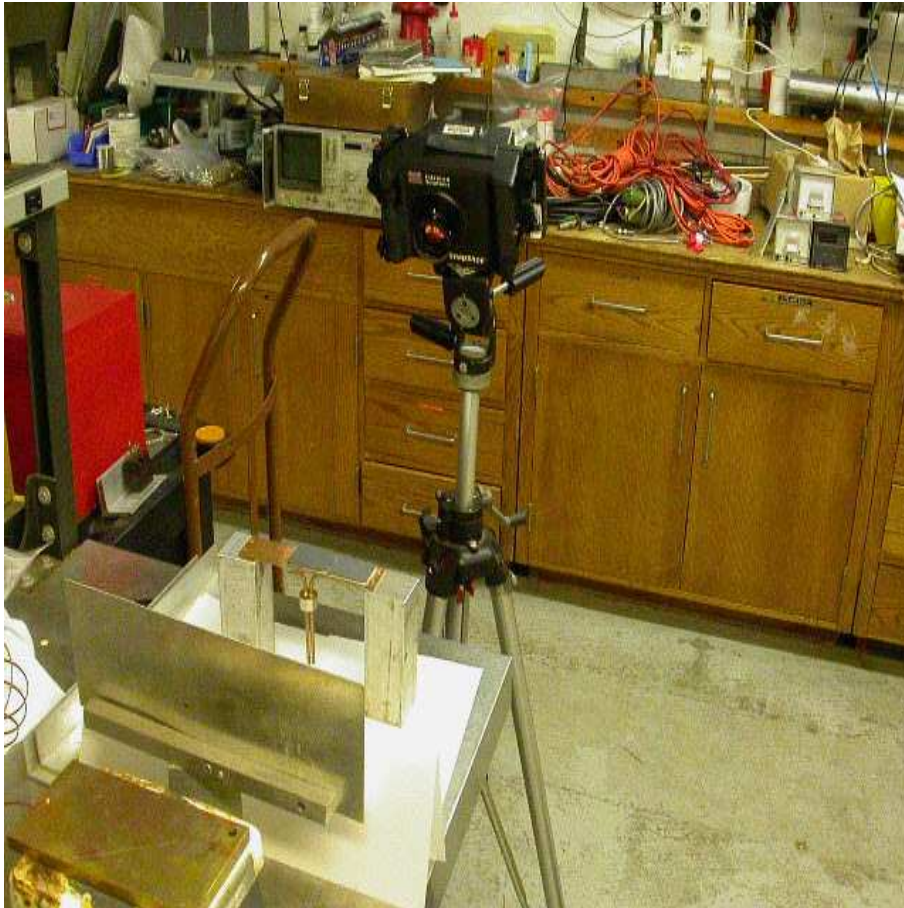
FIG. 2: Testing Setup. Front: heat plate, Middle: tile sample, Back: infrared camera
