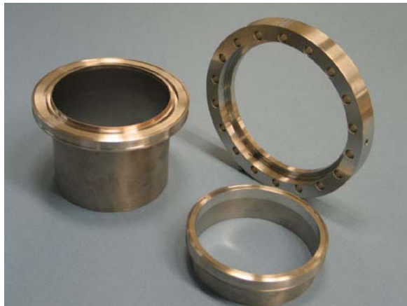
Figure 3: Conflat flanges for 2-cell niobium cavity. Left: vacuum furnace braze; Right: explosion bonding.
