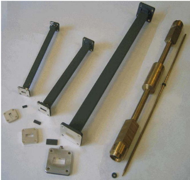
Fig. 1. Transmission lines for four frequency ranges.
