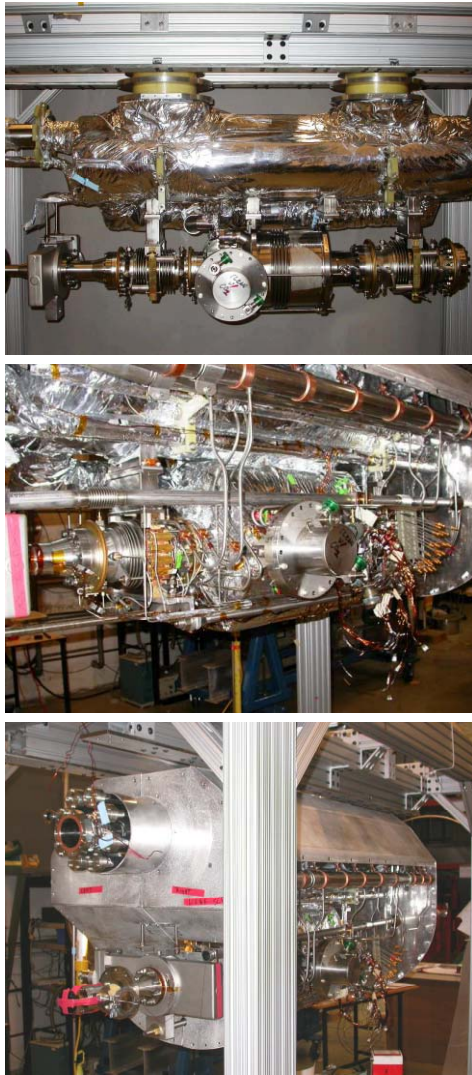
Figure 3: HTC module assembly. Top: Beam line string supported by HGRP. Middle: After adding of 5K and 80K tubing. Bottom: Nearly closed 80K shield.
