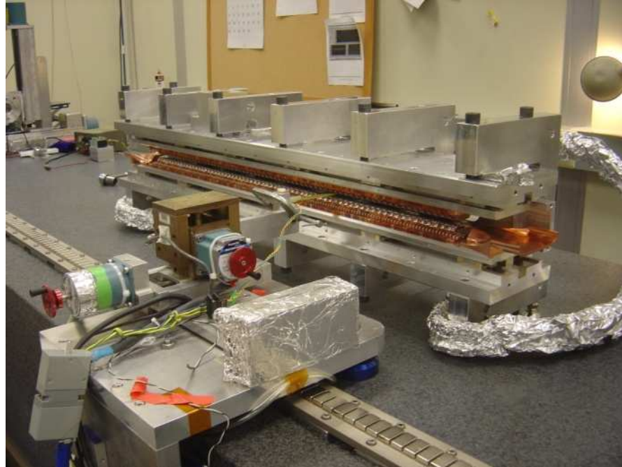
Fig. 13. CHES Compact undulator on magnetic field measurement bench. To provide access to field region over all undulator length, one side plate was temporarily removed and C-clamps were installed.
