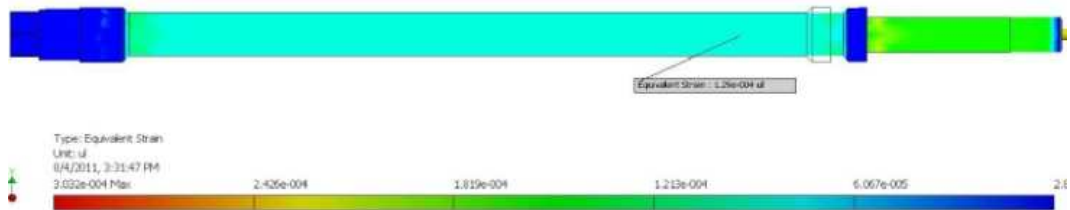
Fig. 8. Drive rod stress analysis. ANSYS predicts the measured 1.29e-5 strain at the gauge location under 5.8 kN applied force.
