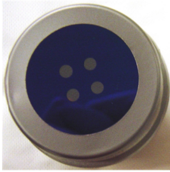
Figure 4: GaAs can easily be masked to reduce halo. The blue area of this cathode is anodized to eliminate emission, while the grey areas have high QE.
