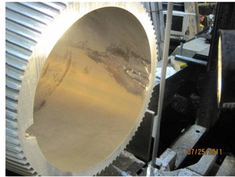
Figure 3: A section of the beam dump [6] before repairs. The left shows where the beam hit, and the right shows the melted aluminium.
