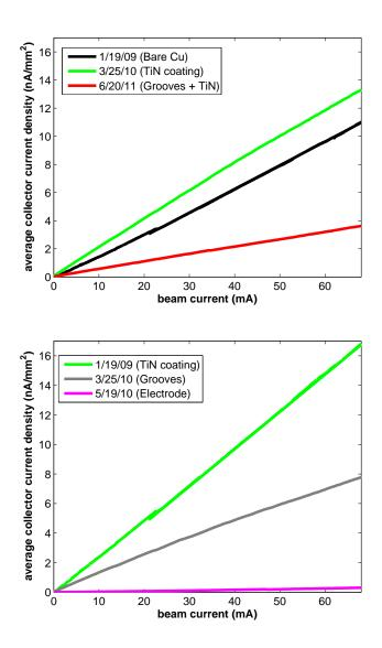
**Figure 5.14:** Wiggler RFA mitigation comparison: 1x45 e+, 2.1GeV, 14ns. Top: 2WA location, bottom: 2WB location. The 2WB location is further downstream in the wiggler straight, and therefore has a slightly higher photon flux.
