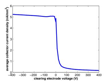
Figure 5.11: Clearing electrode scan: 1x45x1mA e+, 2.1GeV, 14ns
