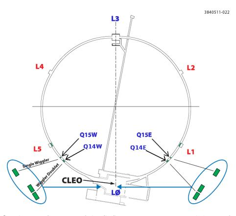
**Figure 1.8:** The reconfiguration of the CESR vacuum system provided space for several electron cloud experimental sections. RFAs are located at L0, Q14E/W, Q15E/W, Q19E, and L3.
