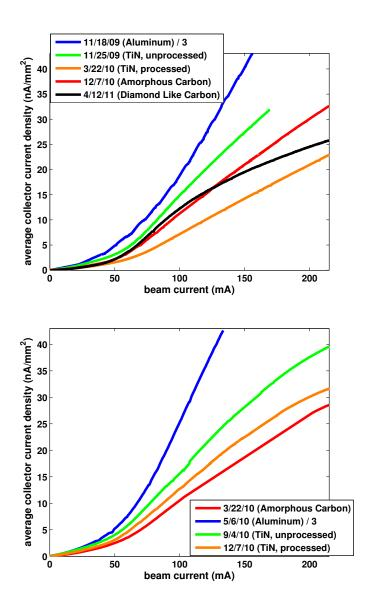
**Figure 2.10:** Comparison of different beam pipe coatings, Q15E (top), and Q15W (bottom) drift RFAs. Plots show average collector signal vs beam current for 20 bunches of positrons with 14 ns spacing, at beam energy 5.3 GeV. Note that the aluminum chamber signals are divided by 3.
