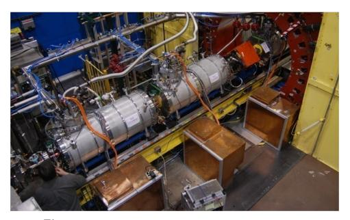
Figure 5.1: Superconducting wigglers in the L0 straight.
