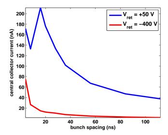
**Figure 2.8:** Central collector signal as a function of bunch spacing, 1x20x3.6mA e<sup>+</sup>, 5.3GeV, in an aC coated chamber at Q15W.
