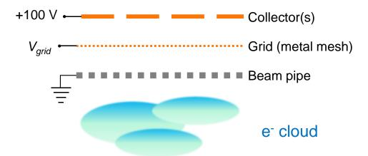
Figure 1.11: Idealized diagram of a retarding field analyzer.
