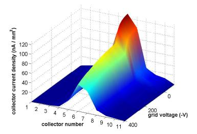
**Figure 2.7:** Voltage scan at high bunch current, 1x20x10 mA e<sup>+</sup>, 5.3 GeV, 14 ns, Insertable II RFA, in a TiN-coated chamber at Q15W.
