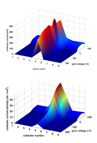
**Figure 3.4:** CESR dipole RFA voltage scans: 1x45x1.25mA e+, 14ns. Top: 5.3 GeV (2010 Gauss); Bottom: 2.1 GeV (790 Gauss). The central collector is no. 5, and the chamber is made of uncoated aluminum.
