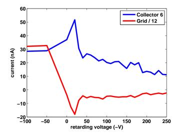
**Figure 5.18:** POSINST simulation showing resonant enhancement, 1x45x1.2 mA e+, 2.1GeV, 14ns, central collector. Compare to Fig. 5.16.
