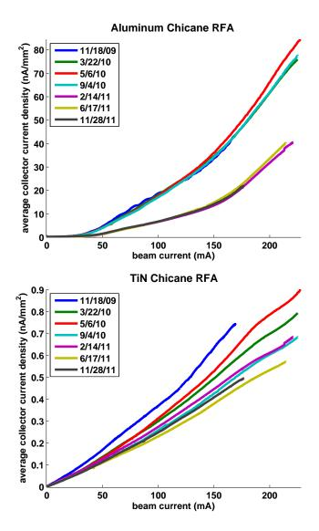
**Figure 3.13:** Long term behavior of chicane dipole RFAs, 1x20 e+, 14 ns, 5.3 GeV. Top: Aluminum chamber, bottom: TiN chamber
