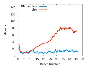
**Figure 1.10:** Bunch-by-bunch beam size and centroid motion, as measured by the X-ray beam size monitor [40].
