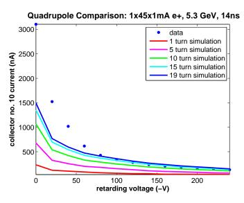
**Figure 4.8:** Quadrupole RFA simulation showing long term cloud buildup: 45 bunches, 1mA/bunch, e+, 5.3 GeV, 14ns
