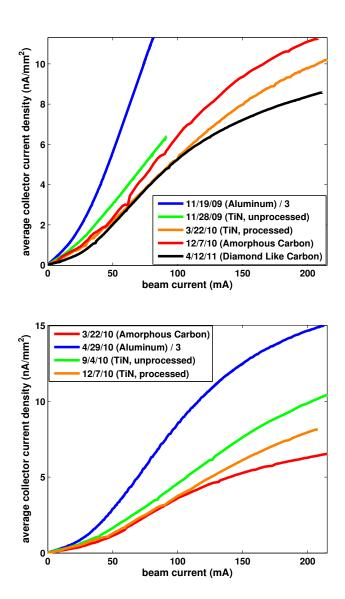
**Figure 2.11:** Comparison of different beam pipe coatings, Q15E (top), and Q15W (bottom) drift RFAs. Plots show average collector signal vs beam current for 20 bunches of electrons with 14 ns spacing, at beam energy 5.3 GeV. Note that the aluminum chamber signals are divided by 3.
