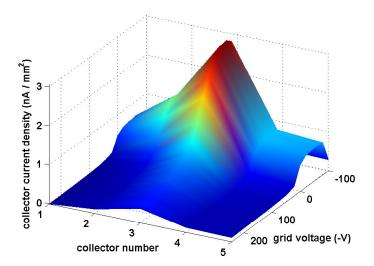
**Figure 2.5:** RFA voltage scan with an "Insertable I" style drift RFA in a Cu chamber, 1x45x1.25 mA e<sup>+</sup>, 14 ns, 5.3 GeV
