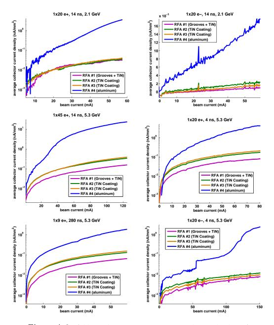
Figure A.2: Additional mitigation comparisons, chicane dipole RFAs
