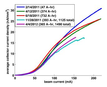
**Figure 2.15:** Performance of Q15E DLC chamber over time, 1x20 e<sup>+</sup>, 5.3GeV, 14ns. Integrated beam doses are given for each measurement. Where two doses are shown, the first is counted from the last CESR down, and the second from the installation of the chamber.
