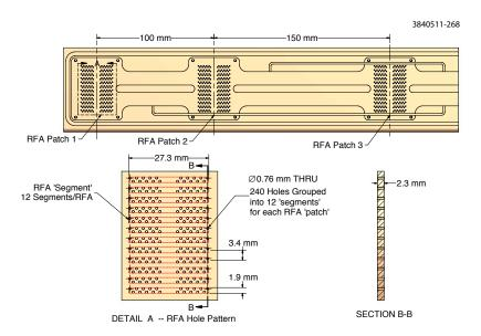
**Figure 5.4:** Small holes are drilled through top beam pipe to allow electrons in the beam pipe drift into RFAs. There are 240 holes for each RFA, and they are grouped into 12 segments to sample transverse EC density distribution.
