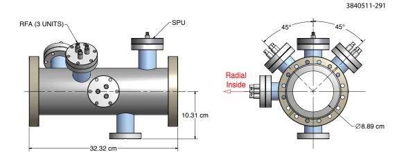
Figure 2.2: Electron cloud diagnostic chamber with NEG thin film coating.
