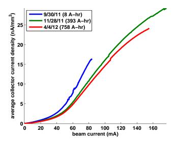
**Figure 2.14:** Processing history in the newer Q15W aC coated chamber, 1x20 e<sup>+</sup>, 5.3GeV, 14ns. Integrated beam doses are given for each measurement.
