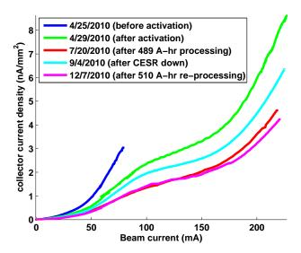
Figure 2.16: NEG RFA comparison, 1x20 e<sup>+</sup>, 5.3GeV, 14ns
