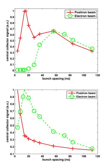
**Figure 3.9:** Central collector signal in a dipole RFA as a function of bunch spacing, for a 20 bunch train with 3.5 mA ( $5.6 \times 10^{10}$  particles) per bunch, at 5.3 GeV. Top: SLAC chicane RFA, bottom: CESR dipole RFA
