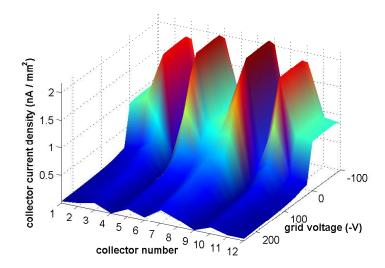
**Figure 5.9:** Grooved wiggler pole center RFA measurement: 1x45x1.25mA e+, 2.1GeV, 14ns looked qualitatively similar (though smaller, due to the difference in photon flux) to the measurements taken in L0. Fig. 5.10 shows an example comparison.
