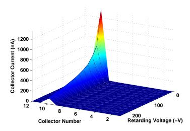
Figure 4.7: Quadrupole RFA simulation: 1x45x1 mA e+, 5.3 GeV, 14ns
