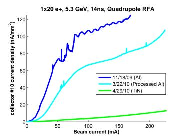
Figure 4.5: Quadrupole mitigation comparison, 1x20 e+, 5.3GeV, 14ns
