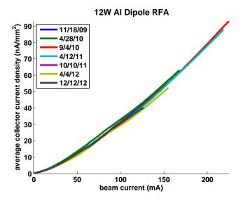
Figure 3.14: Long term behavior of CESR dipole chamber, 1x20 e+, 14 ns, 5.3 GeV
