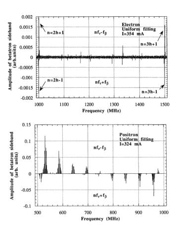
**Figure 1.1:** Evidence of electron cloud induced beam intability at the KEK Photon Factory. The distribution of betatron sidebands was found to be qualitatively different for beams of electrons (top) and positrons (bottom).
