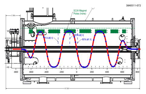
**Figure 5.3:** Three RFAs are built into each SCW RFA beam pipe. A plot of the B-field along the wiggler (red line with blue dots) is superimposed on the drawing of the wiggler. The RFAs are located at three strategic B-field locations, as shown.
