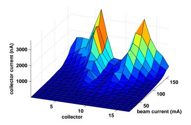
**Figure 3.17:** Simulation of the bifurcation of peak cloud density: 1x20 e+, 5.3GeV, 14ns. Compare to Fig. 3.6
