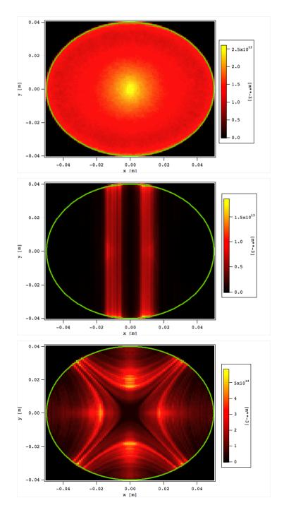
Figure 1.3: Cloud density distributions (averaged over a full turn) in different magnetic fields: drift (top), dipole (middle), and quadrupole (bottom). Plots courtesy M. Furman.
