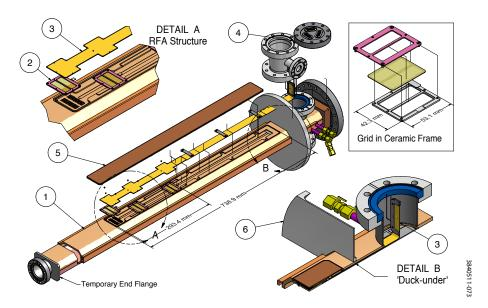
Figure 5.2: Exploded View of a SCW RFA beam pipe Assembly. The key components are: (1) beam pipe top half, housing the RFAs; (2) RFA grids (see upper right inset); (3) RFA collector; (4) RFA connection port; (5) RFA vacuum cover. The 'duck-under' channel, through which the kapton flexible circuit is fed after all heavy welding is complete, is shown in detail B.
