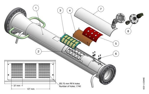
Figure 4.1: Exploded view of the structure of the RFA within a CESR quadrupole beam pipe. The major components of the RFA beam pipe include: (1) Aluminum beam pipe with cooling channels; (2) RFA housing and wiring channels; (3) Retarding grids, consisting of high-transparency gold-coated meshes nested in PEEK frames; (4) RFA collector flexible circuit; (5) Stainless steel backing plate; (6) Wire clamps; (7) RFA vacuum cover with connection port; (8) 19-pin electric feedthrough for RFA connector
