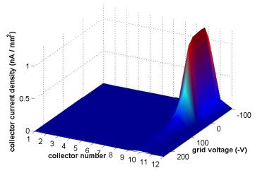
Figure 4.3: Quadrupole RFA voltage scan: 1x45x1.25mA e+, 5.3GeV, 14ns
