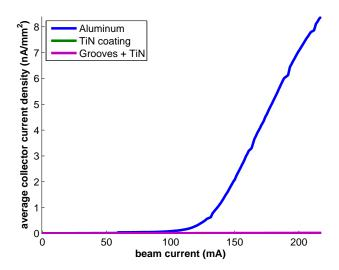
Figure 3.11: Dipole RFA mitigation comparison, 1x20 e-, 5.3GeV, 14ns, 810 Gauss.
