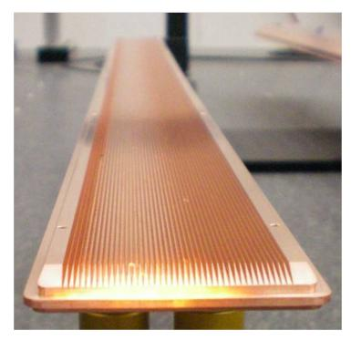
Figure 5.5: Grooved insert for CESR-TA wiggler. The grooves have 2mm depth and 20° angle.
