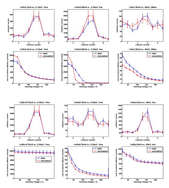
**Figure 2.21:** Comparison of Q15W Al RFA data and simulation, using best fit parameters (Table 2.6). The top plots show the total signal across the 9 RFA collectors (with +50 V on the grid); the bottom plots show the signal in the central three collectors vs retarding voltage.
