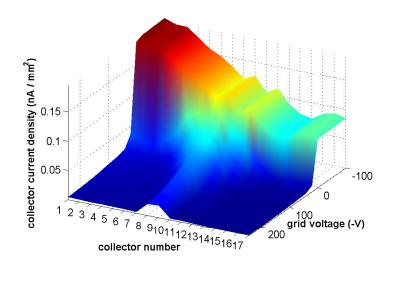
**Figure 3.5:** Chicane dipole RFA voltage scans: 1x45x1.25 mA e+, 14 ns, 5.3 GeV, 810 Gauss. Top: Aluminum chamber; Bottom: TiN-coated chamber. The central collector is no. 9.
