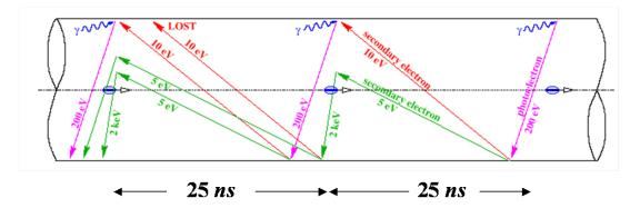
**Figure 1.2:** Illustration of the electron cloud buildup process (in the LHC), courtesy F. Ruggerio.
