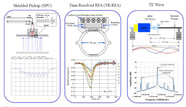
Figure 1.9: Other EC measurement techniques employed at CESR-TA, courtesy J. Sikora.
