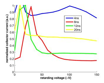
**Figure 5.17:** Resonant spike location at different bunch spacings, 1x45x1.25 mA e+, 5GeV. Only the signal in the central collector is plotted
