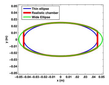
**Figure 2.24:** Comparison of possible chamber shapes in POSINST. Most simulations presented here used the "thin ellipse" shape, which matches the dimensions of the chamber, but not the exact geometry.
