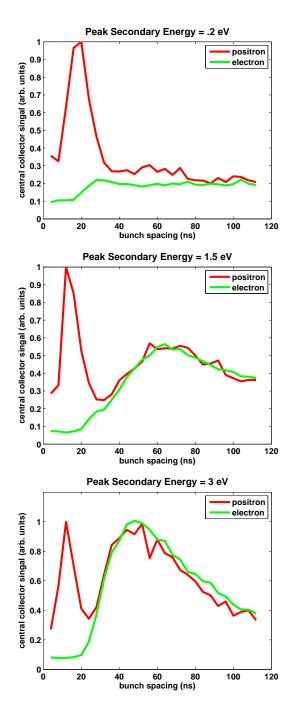
Figure 3.20: Simulation of the multipacting resonances: 1x20x3.5 mA, 5.3GeV, for different "true secondary" energies. Top:  $E_{ts} = .2$  eV, middle:  $E_{ts} = 1.5$  eV, bottom:  $E_{ts} = 3$  eV. The locations of the resonances are very sensitive to this parameter. Compare to Fig. 3.9.
