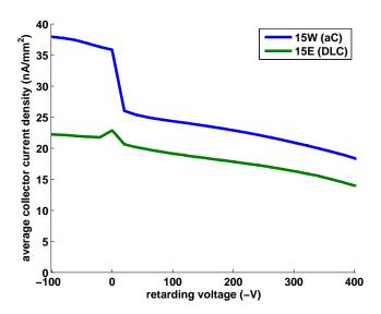
Figure 2.13: Comparison of amorphous and diamond-like carbon at high beam current, 1x20x10mA e<sup>+</sup>, 5.3 GeV, 14 ns.
