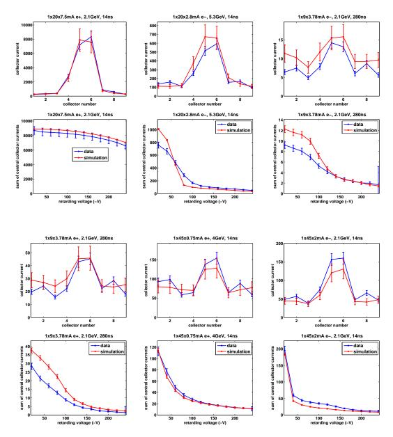
**Figure 2.22:** Comparison of Q15W Al RFA data and simulation, using best fit parameters (Table 2.6). The top plots show the total signal across the 9 RFA collectors (with +50 V on the grid); the bottom plots show the signal in the central three collectors vs retarding voltage.
