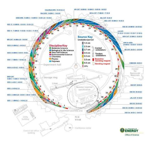
Figure 1.5: Layout of the Advanced Photon Source showing the various experimental stations. Electrons are accelerated in the linac and booster synchrotron, then injected into the storage ring where they are used to generate light.
