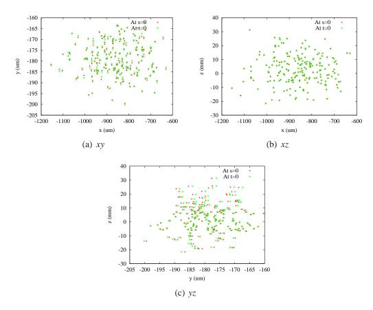
Figure 2.16: x, y, and z coordinates of a bunch at s = 0 and t = 0. The bunch lies on a non-zero closed orbit.
