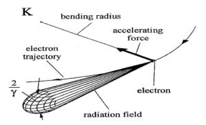
Figure 1.3: A charged particle beam emits a cone of radiation when bent by a dipole magnet. Image source [57].
