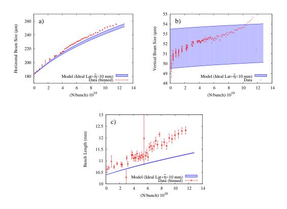
Figure 2.35: Measurements on V15 Managed lattice. (a) horizontal, (b) vertical, and (c) longitudinal beam size versus current for  $e^+$  bunch in CesrTA configured for approximately 55 pm vertical emittance.
