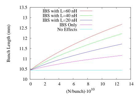
Figure 2.20: Simulated effect on bunch length of PWD in combination with IBS.
