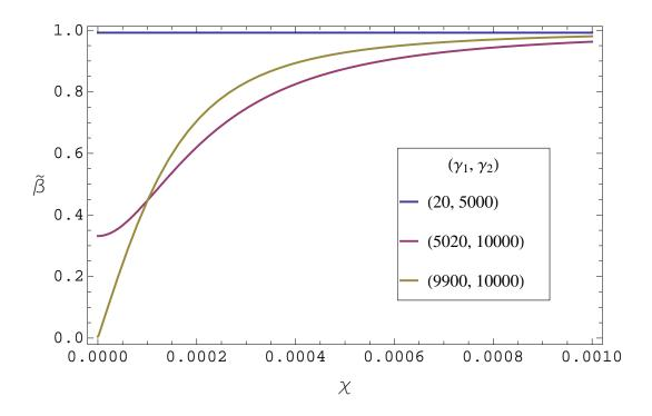
Figure 3.14:  $\tilde{\beta}$ , the velocity of colliding particles in the c.o.m. frame, plotted versus  $\chi$ . When  $\Delta E$  is large, there are no particle pairs with small  $\tilde{\beta}$ .
