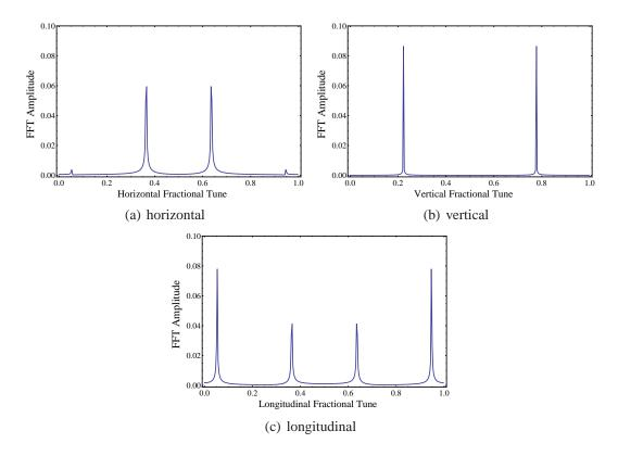
Figure 2.3: Fourier transform of particle motion in x, y, and z over 300 turns. Coupling is evident between the horizontal (a) and longitudinal (c) motion, while the vertical (b) motion is uncoupled.
