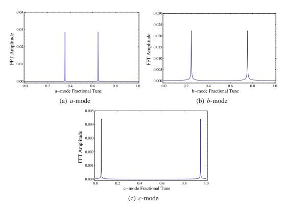
Figure 2.10: Fourier transform of particle motion in a, b, and c over 300 turns.
