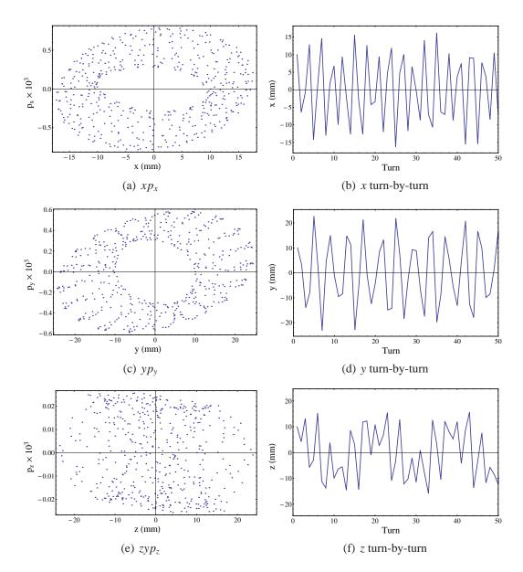
Figure 2.4: Phase space and trajectory of particle tracked through lattice with xy coupling.
