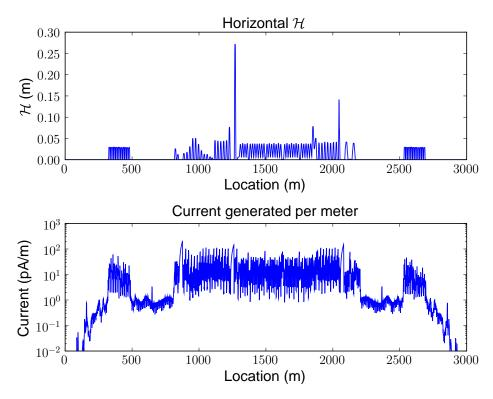
Figure 3.9:  $\mathcal{H}$  and current of scattered particles produced per meter for Cornell ERL.
