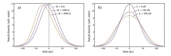
Figure 2.19: Effect of (a) resistive and (b) inductive parts of the longitudinal impedance on the longitudinal profile of the bunch.
