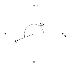
Figure 2.6: Eigenvector  $\lambda = x + iy$  plotted on complex plane. The phase advance of the transfer matrix is  $\Delta \phi$ .
