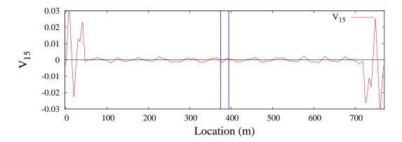
Figure 2.23: xz coupling term  $V_{15}$  along CesrTA with  $V_{15}$  compensation. The blue bands show the locations of the horizontal beam size monitor source points for positrons (374.247 m) and electrons (394.1812 m).
