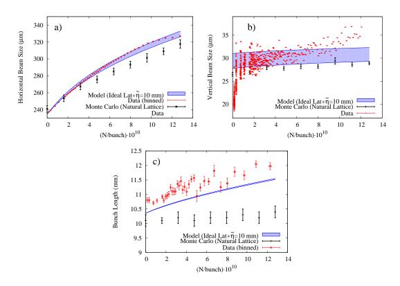
Figure 2.28: (a) horizontal, (b) vertical, and (c) longitudinal beam size versus current for  $e^+$  bunch in conditions tuned for minimum vertical emittance.
