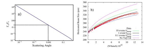
Figure 2.14: (a) Events which occur less than once per damping time are excluded from the calculated growth rate. (b) Equilibrium beam size calculations assuming different cut-offs.
