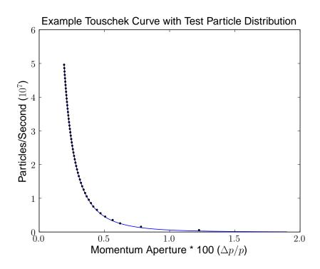
Figure 3.5: Example Touschek curve with test particle distribution used to represent it.
