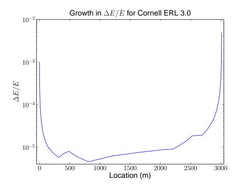
Figure 3.8: Growth  $\Delta E/E$  through linac due to IBS. The injected  $\Delta E/E$  is  $10^{-3}$ . At the end of the linac,  $\Delta E/E$  is  $4.9 \times 10^{-3}$ .
