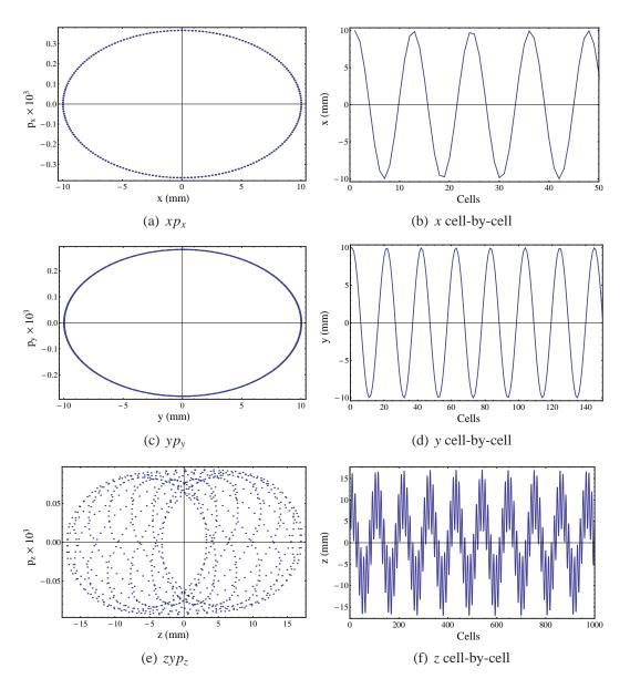
Figure 2.1: Trajectory of particle with initial coordinates (0.01, 0, 0.01, 0, 0.01, 0) tracked repeatedly through a single FODO cell.
