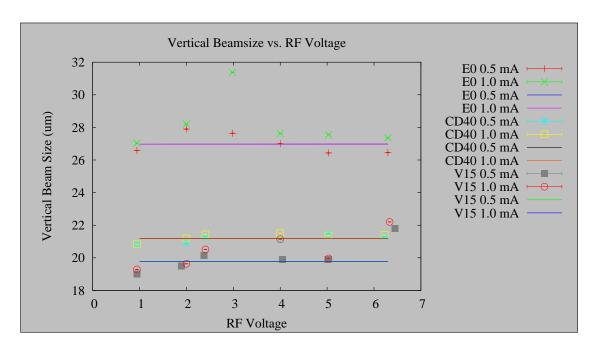
Figure 2.42: Vertical beam size versus RF voltage. The simulation lattices here are ideal with no vertical dispersion. Expected response is flat versus RF voltage.
