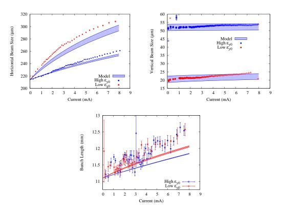
Figure 2.40: Aggregated 2.3 GeV data. (a) horizontal, (b) vertical, and (c) longitudinal beam size versus current. Optics are configured to minimize  $V_{15}$  coupling at the horizontal beam size monitor source point.
