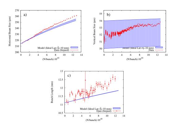
Figure 2.39: (a) horizontal, (b) vertical, and (c) longitudinal beam size versus current for 2.3 GeV  $e^+$  bunch in CesrTA configured for approximately 54 pm vertical emittance.
