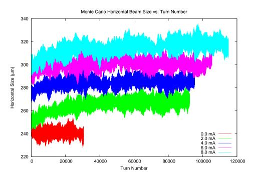
Figure 2.18: Horizontal beam size versus turn from Monte Carlo simulation that incorporates intrabeam scattering. The equilibrium distribution from the lower current runs are used to seed the higher current runs.
