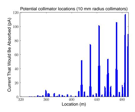
Figure 3.10: Histogram of the current of particles scattered in TA and lost in SA that would be caught by a collimator at the given location. The horizontal coordinate spans the TA region.
