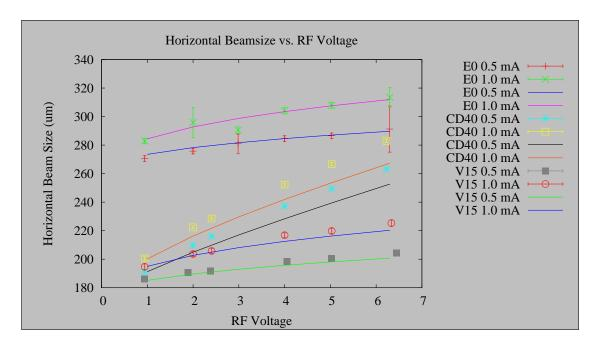
Figure 2.41: Horizontal beam size versus RF voltage. Both V15 tilt and IBS effects are observed in this data.
