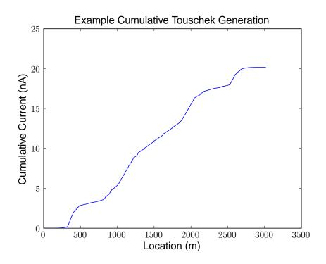
Figure 3.4: Cumulative generation of scattered particles.
