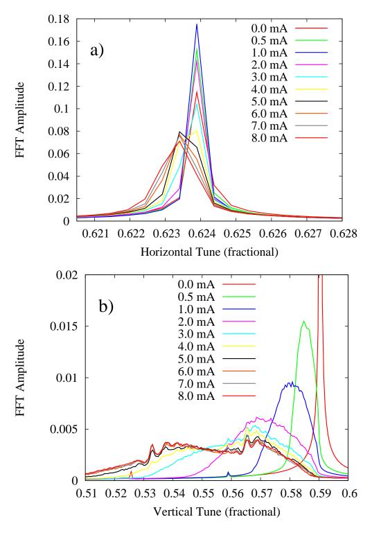
Figure 2.26: Monte Carlo simulation of direct space charge showing the (a) horizontal and (b) vertical tune spread predicted for various currents. The conversion factor between mA and particles/bunch in CesrTA is  $1.6 \times 10^{13}$  seconds/Coulomb.
