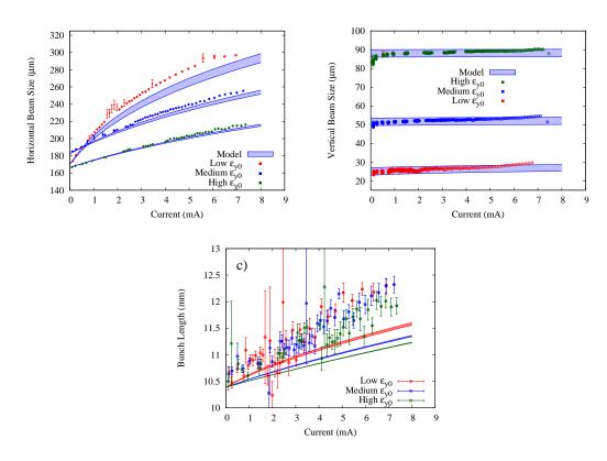
Figure 2.37: Measurements on V15 Managed lattice. Aggregated (a) horizontal, (b) vertical, and (c) longitudinal data comparing  $e^+$  in minimum emittance conditions and conditions where the zero current vertical emittance was blown up using closed coupling and dispersion bumps.
