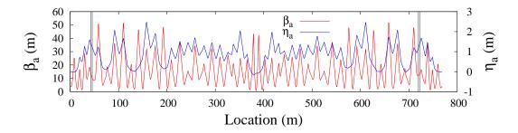
Figure 2.21: CesrTA design a-mode (horizontal-like)  $\beta$  and dispersion  $\eta$ . The gray vertical bars indicate the locations of CesrTA's four RF cavities. Horizontal dispersion in the RF cavities is about 1 m.
