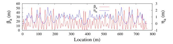
Figure 2.29: CesrTA design a-mode (horizontal-like)  $\beta$  and dispersion  $\eta$ .
