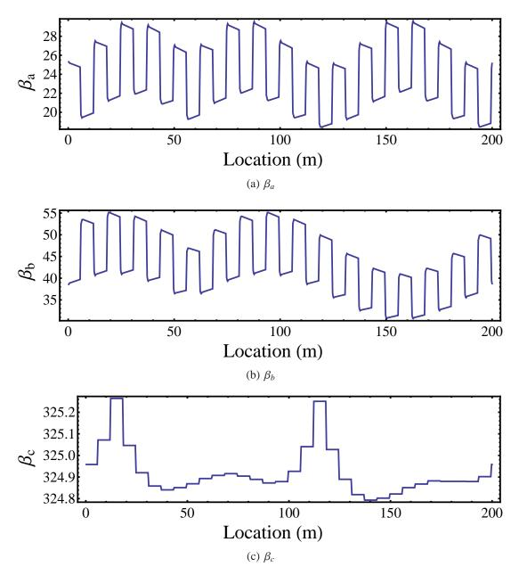
Figure 2.12: Normal mode  $\beta$ -functions calculated from eigen-decomposition of the 1-turn transfer matrix. The lattice elements are not symmetric about s=0 m.
