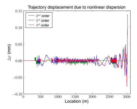
Figure 3.2: Displacement of trajectory of particle with +10 MeV/c momentum defect due to  $2^{nd}$ ,  $3^{rd}$ , and  $4^{th}$  order dispersion. The beam pipe diameter is 13 mm.
