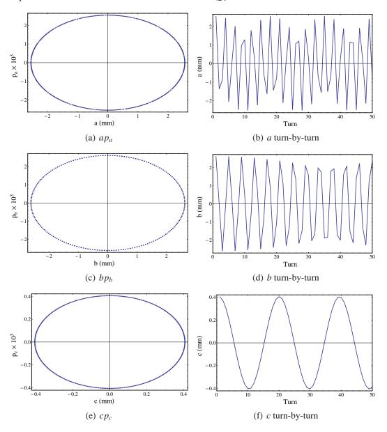
Figure 2.9: Phase space and trajectory in the eigenbasis of the machine.
