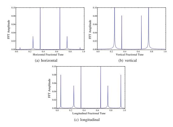
Figure 2.5: Fourier transform of x, y, and z particle motion over 500 turns in demonstration lattice with horizontal-vertical coupling.
