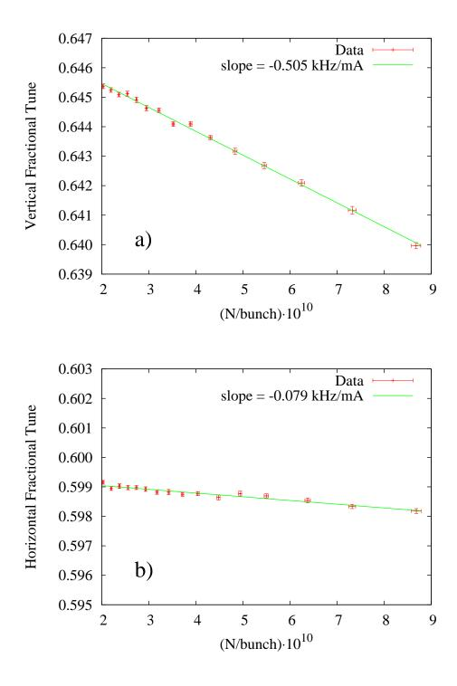
Figure 2.24: Fractional coherent tune versus current for (a) the vertical and (b) the horizontal plane. The resolution of the measurement is  $10^{-4}$ . The revolution frequency is 390.1 kHz.
