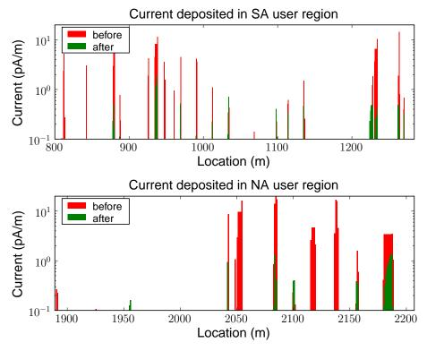
Figure 3.11: Results of collimating Cornell ERL to reduce current of scattered particles deposited into user regions. The red bars are before collimation, and the green bars after collimation. All green bars are below the 3 pA/m threshold.
