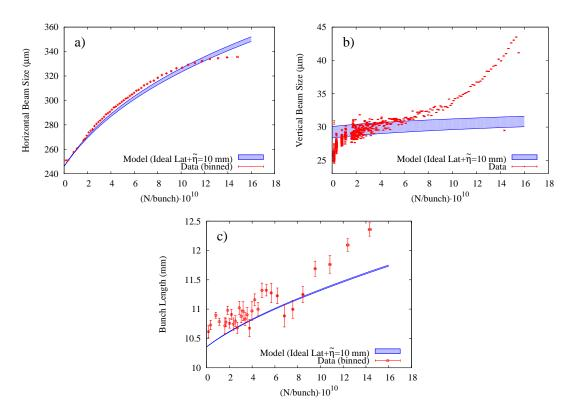
Figure 2.31: (a) horizontal, (b) vertical, and (c) longitudinal beam size versus current for  $e^-$  bunch in conditions tuned for minimum vertical emittance. An uninitialized transverse feedback system was mistakenly turned on during this run. It drove the coherent tunes onto the (1, -1, 1, 0) resonance line at currents  $5.6 \times 10^{10}$  above part/bunch.
