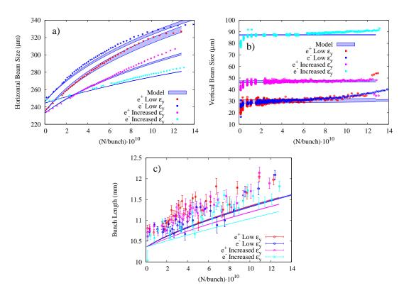
Figure 2.33: Aggregated (a) horizontal, (b) vertical, and (c) longitudinal data comparing  $e^+$  and  $e^-$  in minimum emittance conditions and conditions where the zero current vertical emittance was blown up using closed coupling and dispersion bumps.
