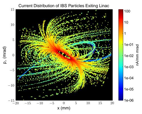
Figure 3.12: Horizontal phase-space distribution of scattered particles at the end of the linac. The total current of particles laying outside 10 sigma of the beam is 413 nA, compared to a beam current of 100 mA. The radius of the beam pipe at this part of the accelerator is 1.95 cm. This data was run on the uncollimated lattice.
