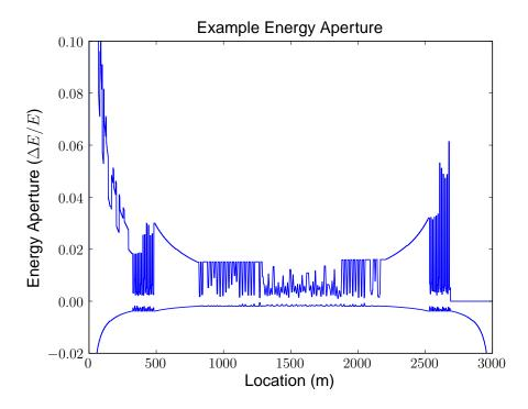
Figure 3.3: Example energy aperture from CERL lattice version 3.0. The positive aperture is determined entirely by beam pipe collisions. The negative aperture is dominated by stopping during deceleration.
