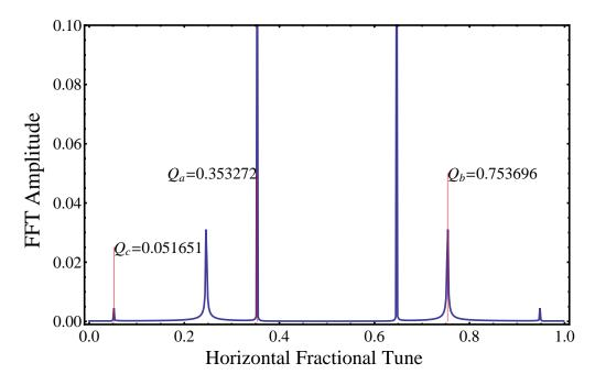
Figure 2.8: Comparing horizontal Fourier transform of particle motion in fully coupled machine to the eigen mode tunes calculated from eigenvalues of the 1-turn map.
