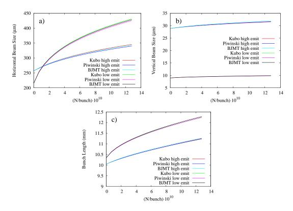
Figure 2.15: Comparing (a) horizontal, (b) vertical, and (b) longitudinal beam size versus current for three different IBS formalisms. The high emittance lattice has  $\epsilon_{x0} = 4.6$  nm·rad,  $\epsilon_{y0} = 14.3$  pm·rad, and  $\sigma_{z0} = 10.0$  mm. The low emittance lattice has  $\epsilon_{x0} = 2.8$  nm·rad,  $\epsilon_{y0} = 1.5$  pm·rad, and  $\sigma_{z0} = 10.3$  mm.
