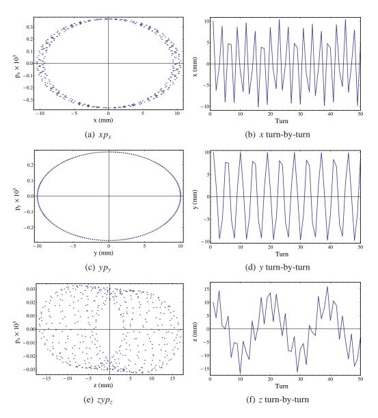
Figure 2.2: Trajectories in phase space of particle with initial coordinates (0.01 m, 0, 0.01 m, 0, 0.01 m, 0) tracked 500 turns through the demonstration lattice.
