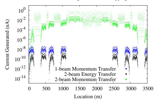
Figure 3.15: Touschek rate for scattering rate between overlapping beams of different energy. The self-scattering rate for the higher energy beam is also plotted for comparison.
