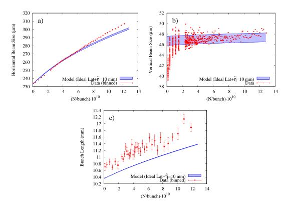
Figure 2.30: (a) horizontal, (b) vertical, and (c) longitudinal beam size versus current for  $e^+$  bunch with increased zero current vertical emittance.
