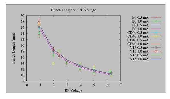
Figure 2.43: Bunch length versus RF voltage. The primary effect see here is the change in bunch length due to change in RF cavity voltage.
