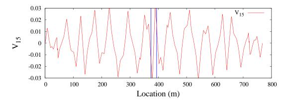
Figure 2.22: xz coupling term  $V_{15}$  along CesrTA. The blue bands show the locations of the horizontal beam size monitor source points for positrons (374.247 m) and electrons (394.1812 m).
