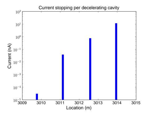
Figure 3.7: Current per decelerating cavity of scattered particles stopping at the end of the linac. The design energy at the end of the linac is 10 MeV. Each cavity decelerates the beam by 13 MeV.
