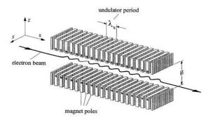
Figure 1.4: In an undulator, a series of bends causes the particle beam to emit an intense pulse of light. Image source [57].
