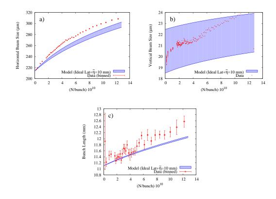
Figure 2.38: (a) horizontal, (b) vertical, and (c) longitudinal beam size versus current for 2.3 GeV  $e^+$  bunch in CesrTA configured for approximately 6 pm vertical emittance.
