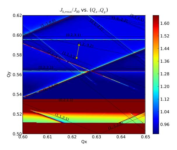
Figure 2.27: Simulated tune scan based on a lattice model that includes magnet misalignments and corrector magnet settings determined according to our emittance tuning procedure. The yellow line shows how the coherent tunes increase as a bunch decays from  $1.3 \times 10^{11}$  down to to  $1.6 \times 10^9$  particles.
