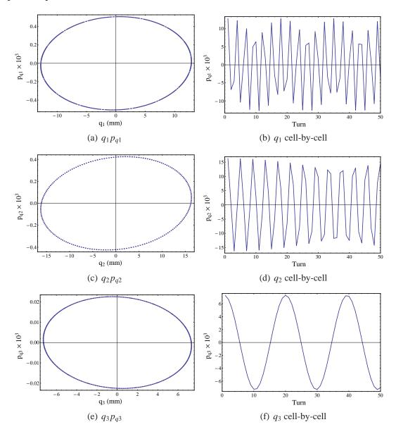
Figure 2.11: Trajectory in normal coordinates of particle with initial lab frame coordinates (0.01 m, 0, 0.01 m, 0, 0.01 m, 0). Particle is tracked for 500 turns.
