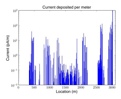
Figure 3.6: Current per meter of scattered particles striking beam pipe. The current at the end of the linac peaks at 2230 pA/m due to the  $1/\gamma(s)$  dependence in Eqn. (3.67).
