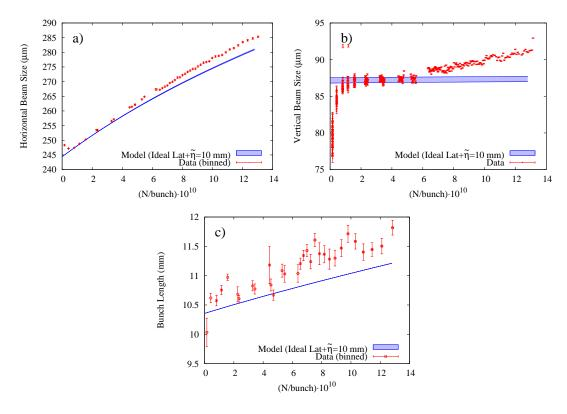
Figure 2.32: (a) horizontal, (b) vertical, and (c) longitudinal beam size versus current for  $e^-$  bunch with increased zero current vertical emittance. An uninitialized transverse feedback system was mistakenly turned on during this run. It drove the coherent tunes onto the (1, -1, 1, 0) resonance line at currents above  $5.6 \times 10^{10}$  part/bunch.
