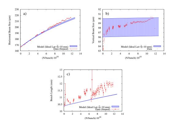
Figure 2.36: Measurements on V15 Managed lattice. (a) horizontal, (b) vertical, and (c) longitudinal beam size versus current for  $e^+$  bunch in CesrTA configured for approximately 160 pm vertical emittance
