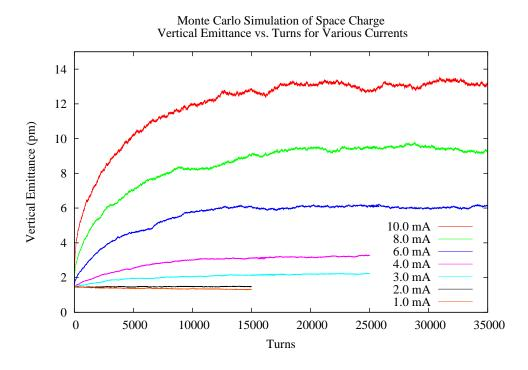
Figure 2.25: Monte Carlo simulation of direct space charge. The vertical beam size equilibrates to a larger value as current is increased.
