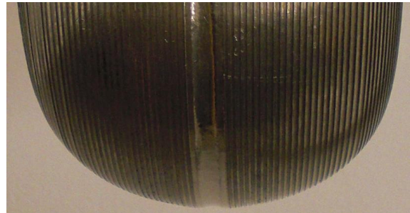
Figure 4: Photo of 1.3 GHz Niobium cavity with machined grooves to increase cooling. The grooves are 1.2 mm deep at 1 mm spacing.
