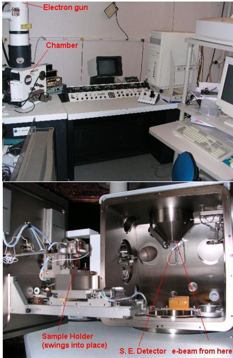
Figure 4: Scanning electron microscope. Above: the instrument. Below: inside the chamber with the door open. Note that the secondary electron detector is off to the side, rather than directly above (the primary electrons come from directly above).
