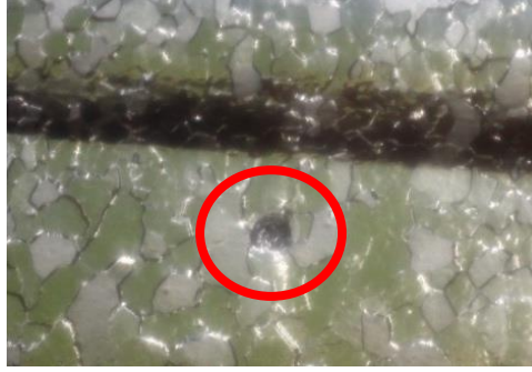
Figure 7.4: A defect (bump) at the quench location in AES022 obtained via optical inspection.
