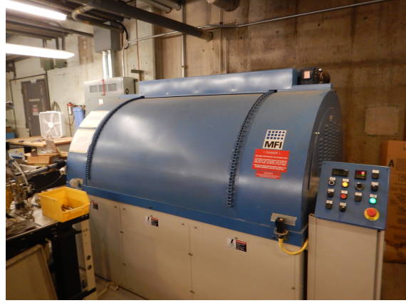
(b) Picture of the Cornell tumbler for centrifugal barrel polishing (CBP).
