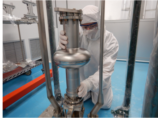
(b) Picture of a cavity being assembled on the single-cell test insert.
