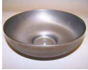
Figure 4.1: A pressed niobium half-cell before receiving rough trimming and being welded into a dumbbell structure.
