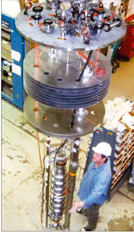
Figure 4.8: ERL 7.1 on experimental insert prior to vertical test.
