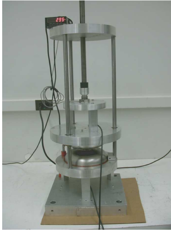
Figure 4.5: A dumbbell inside the frequency measurement apparatus, used to determine how much material to trim from the equator region so that after welding the cavity has the proper resonant frequency. The screw allows the same force to be applied to each dumbbell, preventing unequal loading which could effect the measured resonant frequency. Image reproduced from [SC12].
