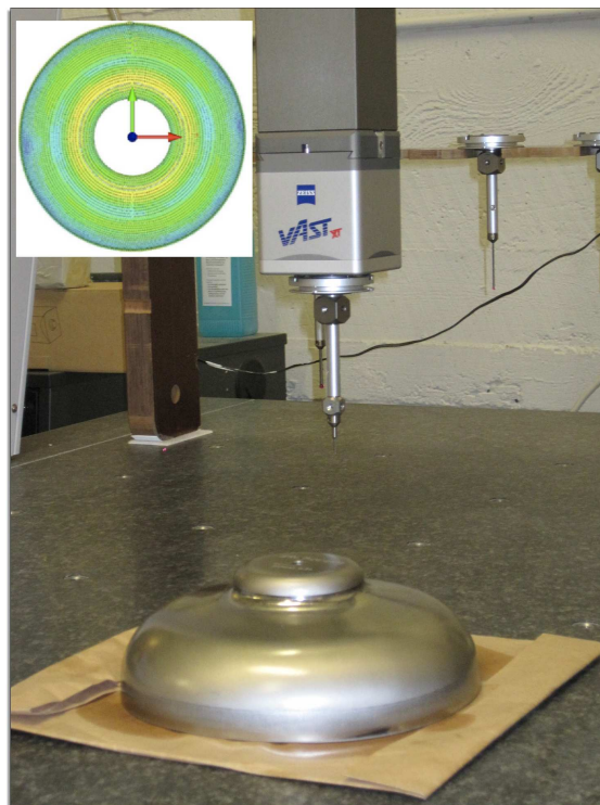
Figure 4.2: Apparatus used to measure cell shape profiles. The stylus contacts the niobium surface and can either measure distances along a profile line or raster over the entire surface to make a 3D representation of the cavity. Inset at top left is a topographical map of cell shape fabrication accuracy.
