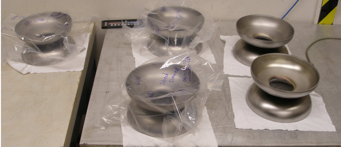
Figure 4.4: Cells after being welded to form dumbbells. These cells were subsequently measured to determine final trimming, and welded into a full cavity.
