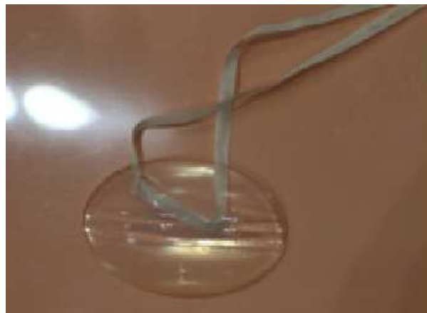
Figure 5.13: One silicone solidified with string after being pulled out from the pits cavity.
