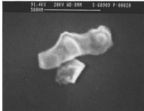
Figure 4 : Residue after a twelve day submersion in de-ionized water on A2-39 (left) and an Aluminum contaminant found on A1-39.
