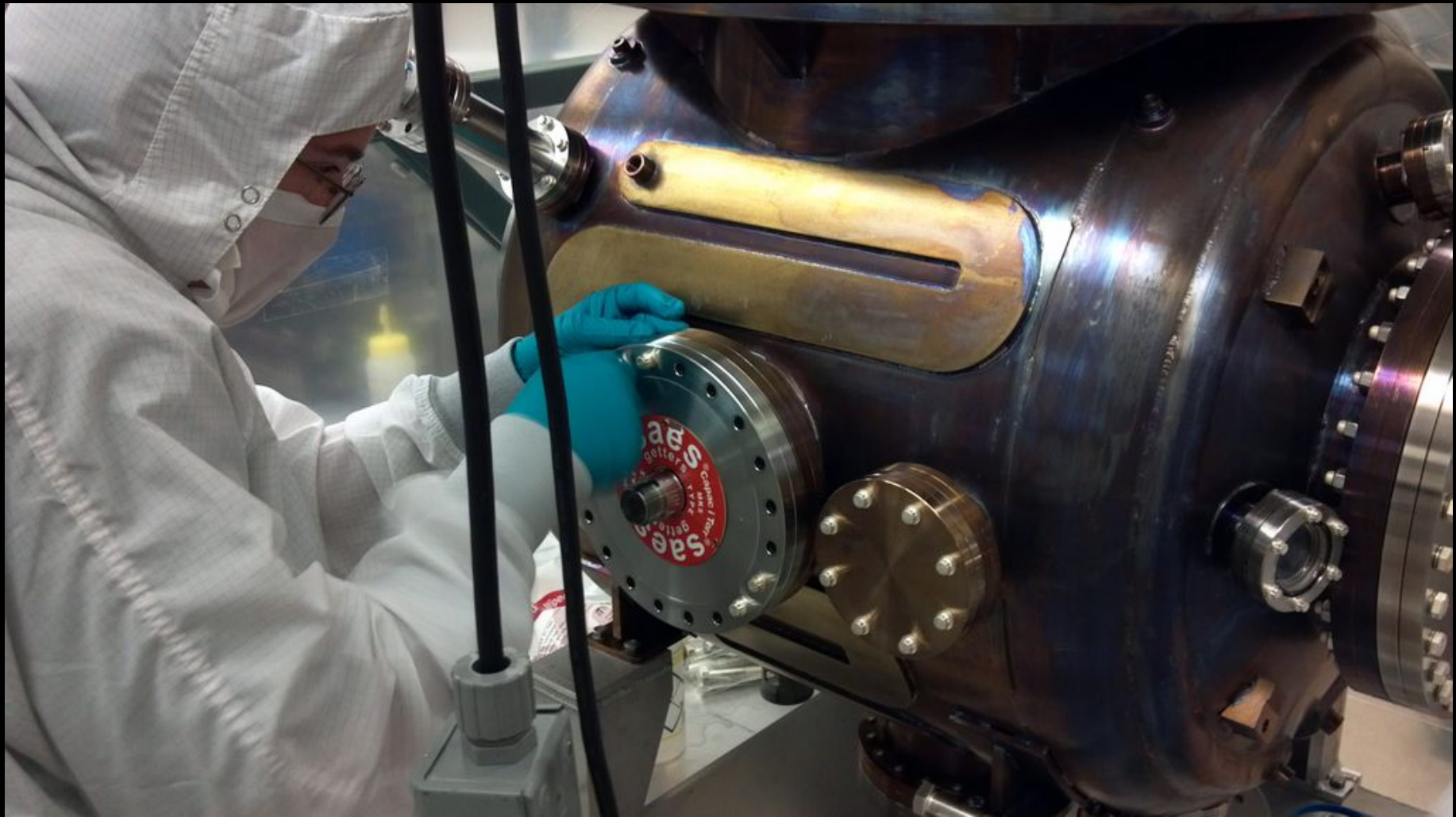
Installing the non-evaporable getter pump.
