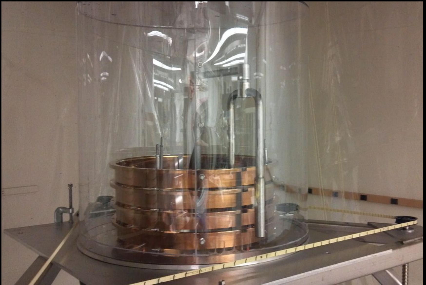
High pressure rinsing protection rings.
