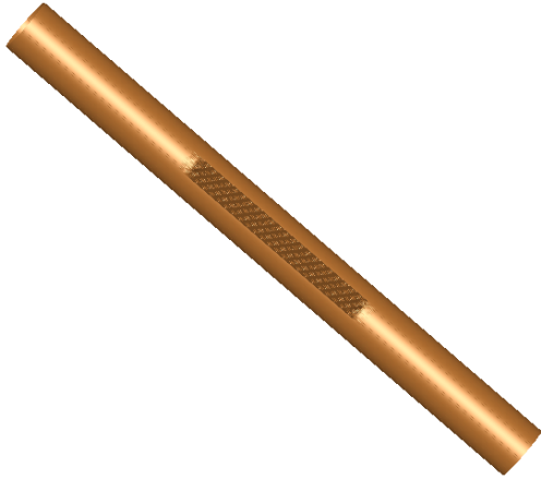
Figure 4: smooth-grooved-smooth beam-pipe lengthwise view from VORPAL simulation
