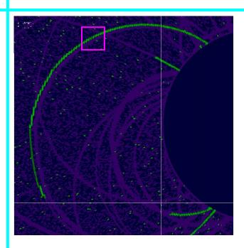
Ionization is spread across the cells. Previously, ionization was created only where the track crossed the central radius.
