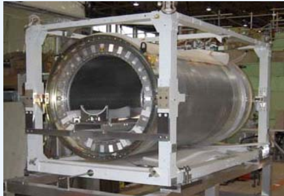
1.5 Tesla, 90 cm bore, magnet
