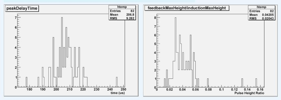
Average pulse delay time is 207  $\mu s$  with  $\sigma$  = 9.3  $\mu s$
