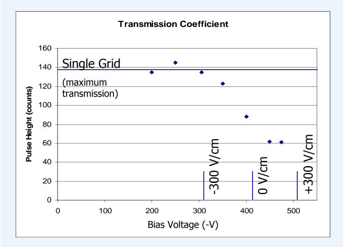
Transmission coefficient of electrons through double field cage termination wires using Micromegas
