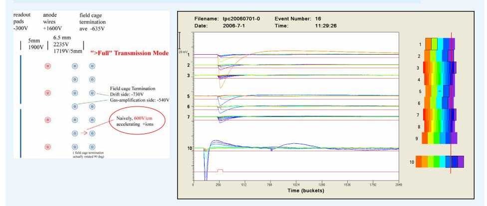
Pulse still observed on field cage termination; decreased signal to noise ratio makes pattern-recognition difficult
