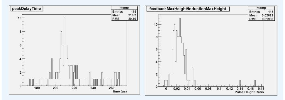
Average delay time is 216  $\mu$ s with  $\sigma = 21 \ \mu$ s
