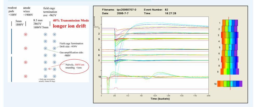
Change the ion drift distance to see if the pulse changes accordingly
