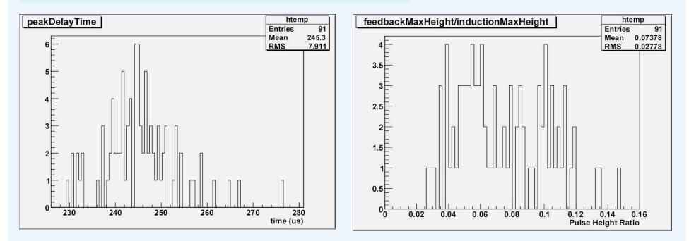
Average pulse delay time is 245  $\mu$ s with  $\sigma$  = 7.9  $\mu$ s (5mm – 202  $\mu$ s) Pulse delay time increase of 21% (40% drift distance increase) Average relative pulse height is 7.4% (5mm – 6.0%)
