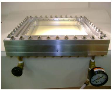
First test, atoxygen overpressure,~ 4 cc/hour/panel.
