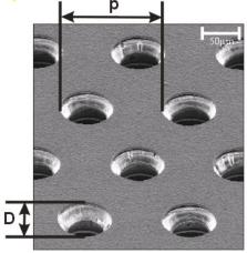
P~140 μm D~60 μm Micromegas: micromesh sustained by 50µm pillars, multiplication between anode and mesh, one stage
